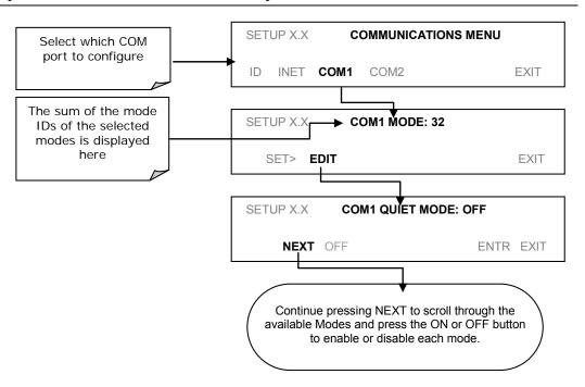
Figure 6-1: COM1[2] – Communication Modes Setup
